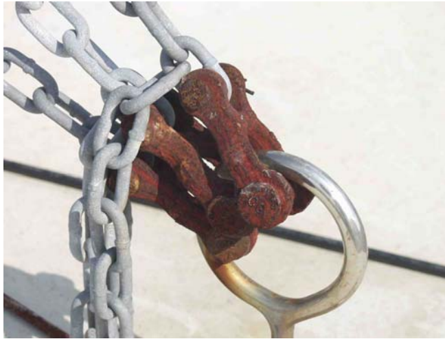
Figure 16 Example of a Rusty Joint
