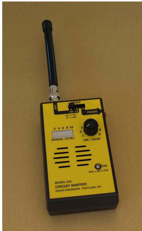
Figure 67 Circuit Sniffer Used to Locate On-Site Sources
