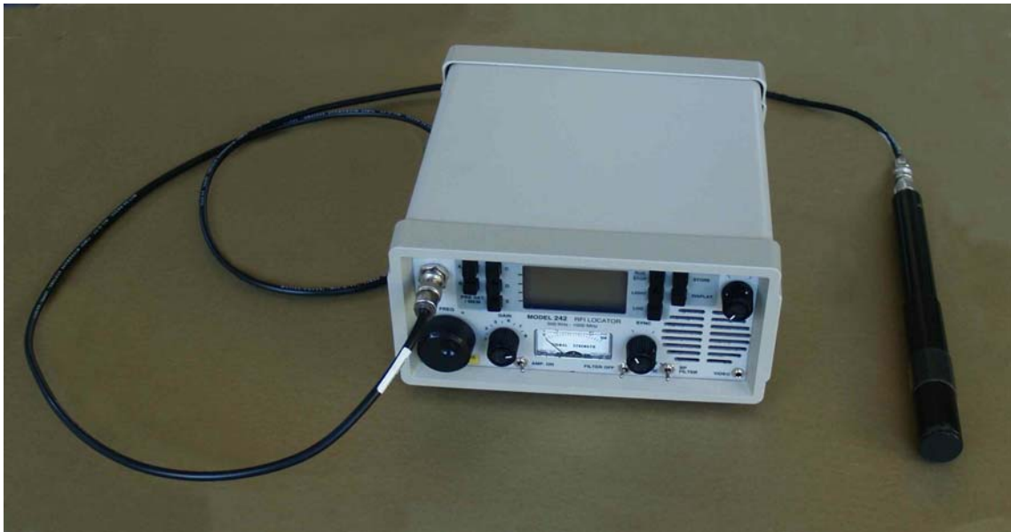
Figure 65 Radar Engineers Noise Receiver with Probe
