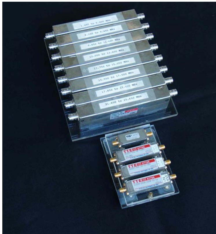
Figure 59 Example of Band-pass Filters
