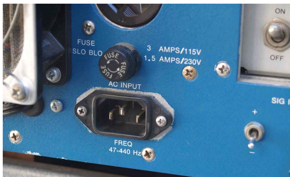
Figure 47 Power Connector that Complies with BFG Principles
