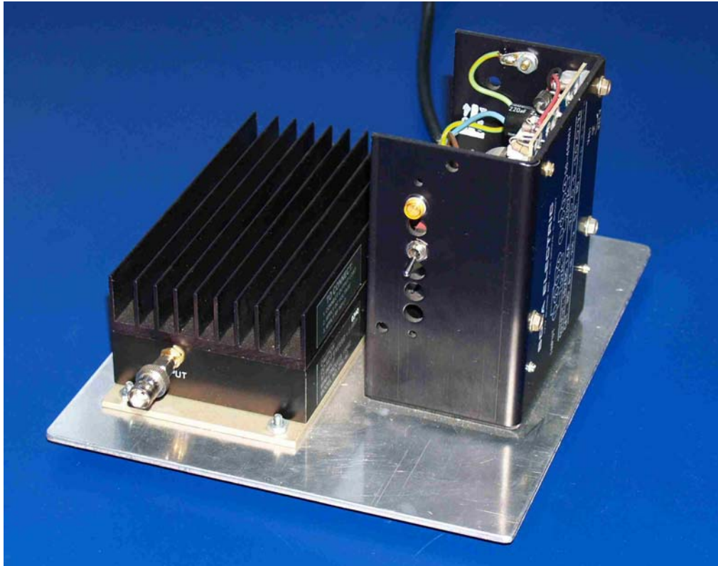
Figure 62 Example of a Preamplifier for the UHF Band
