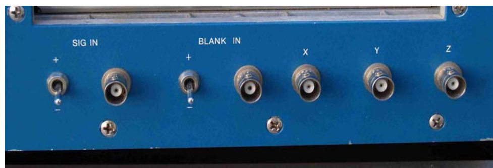
Figure 48 Coax Feed Bulkhead Connectors that Comply with BFG Principles
